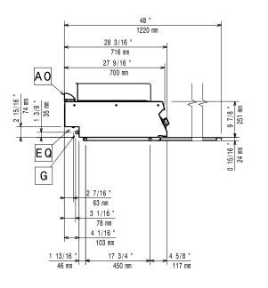
EQ = Equipotential screwG = Gas connection
